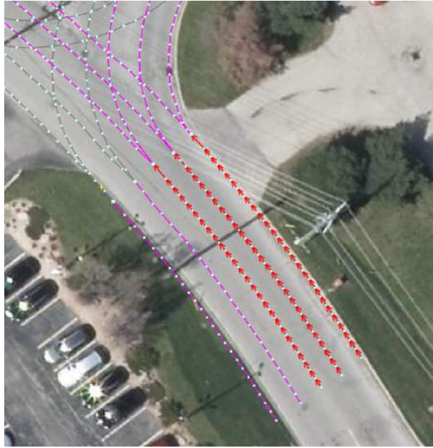
Figure 2.5: Lanelet with connections shown in JOSM
