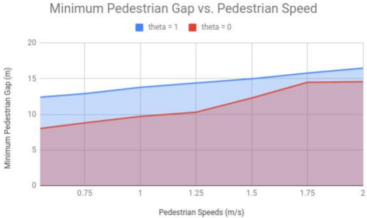
Figure 4.3: Pedestrians walking speeds vs. minimum gap distance for ego to cross
